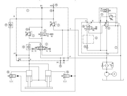
The above scheme refers to PBTC-1016-NO execution coupled with Atos normally open prefilling valves, pos.  $\textcircled{\textbf{6}}$
