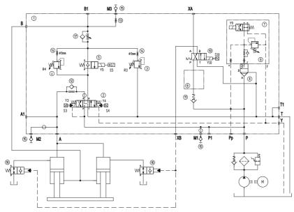
The above scheme refers to PBTC-1616-NO execution coupled with Atos normally open prefilling valves, pos. 6
